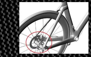
Internal cabling ready for electronic shifting - ICRS
